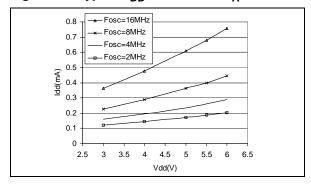
Figure 68. Typical  $I_{DD}$  in WAIT at  $T_A$ =25°C
