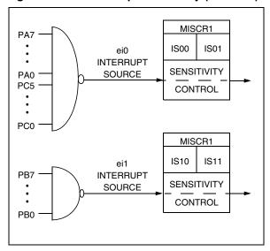
Figure 30. Ext. Interrupt Sensitivity (EXTIT=1)
