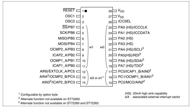
Figure 3. 32-Pin SDIP Package Pinout
