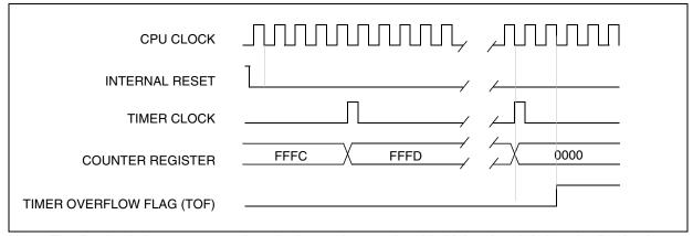
**Note:** The Device is in reset state when the internal reset signal is high, when it is low the Device is running.
