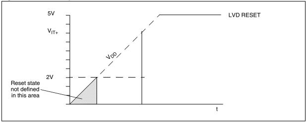
**Note:** When the LVD is enabled, the MCU reaches its authorized operating voltage from a reset state. However, in some devices, the reset signal may be undefined until  $V_{DD}$  is approximately 2V. As a consequence, the I/Os may toggle when  $V_{DD}$  is below this voltage.
