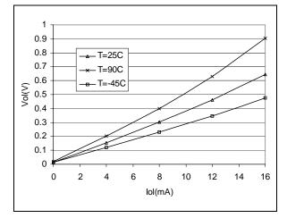
Figure 82. Typ. V<sub>OL</sub> at V<sub>DD</sub>=2.7V (standard)
