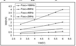
Figure 69. Typ.  $I_{DD}$  in SLOW-WAIT at  $T_A$ =25°C
