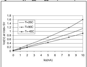
Figure 81. Typ. V<sub>OL</sub> at V<sub>DD</sub>=3V (high-sink)
