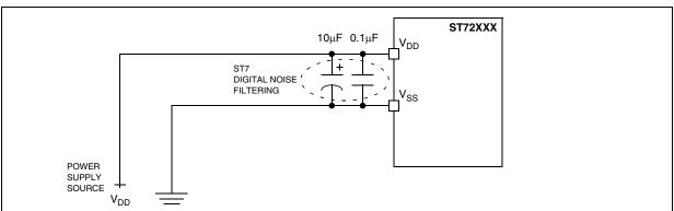
1. The suggested 10µF and 0.1µF decoupling capacitors on the power supply lines are proposed as a good price vs. EMC performance tradeoff. They have to be put as close as possible to the device power supply pins. Other EMC recommendations are given in AN1709.
