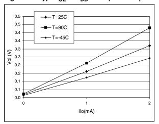
Figure 83. Typ. V<sub>OL</sub> at V<sub>DD</sub>=5V (high-sink)
