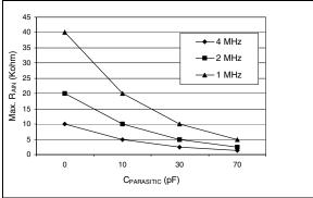
Figure 98. Recommended C<sub>AIN</sub>/R<sub>AIN</sub> values<sup>3)</sup>
