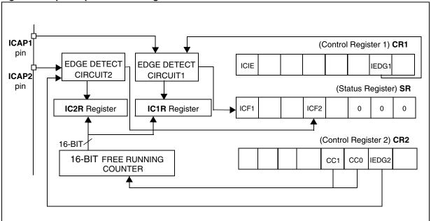
Figure 40. Input Capture Timing Diagram
