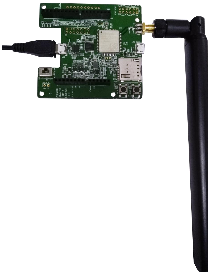
Figure 14: BC66-TE-B Kit Assembly
